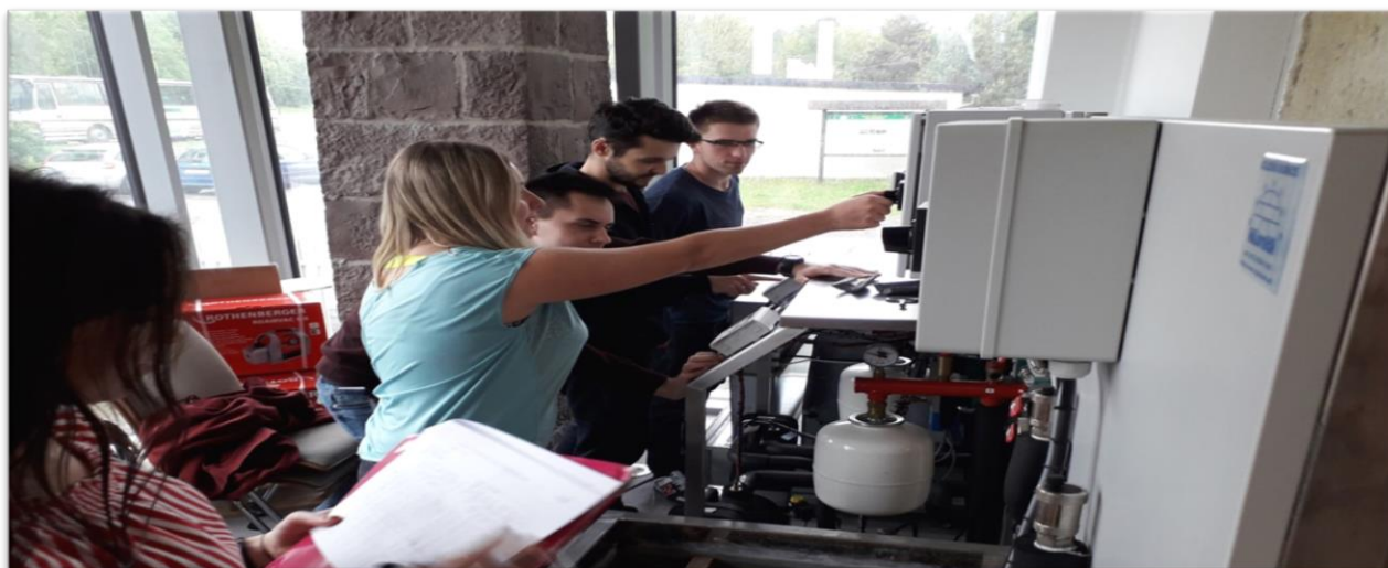
Figure 2. Students during measurements of heat pump efficiency
